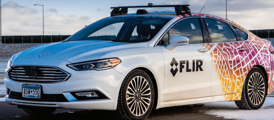
FIGURE 1: VSI test car equipped with the FLIR ADK, radar and neural network for AEB pedestrian detection
